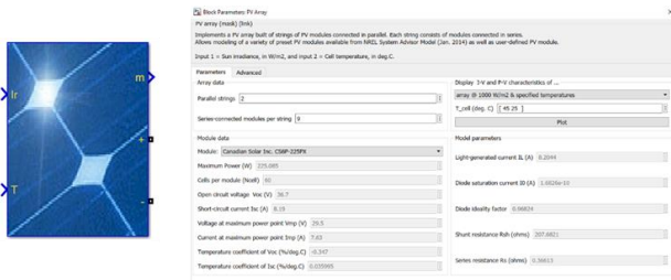
Figure 1- PV Array block (left) and block's data (right).
